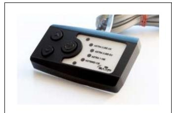
The control panel has an on/off button and an UP and a Down button. Pressing the main on/off button will wake the antenna. It will then go to the last satellite that it tracked. After waking the antenna, you can alter the satellite you would like to track by using the UP or Down button until your desired satellite is lit by the blue LED light. Pressing the on/off again button will shut it down.
