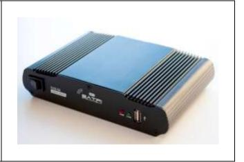
Software updates, firmware or satellite frequencies can be emailed to you. They should be downloaded to a blank USB stick and inserted into the USB port. The unit should then be switched on and the update will happen automatically.
